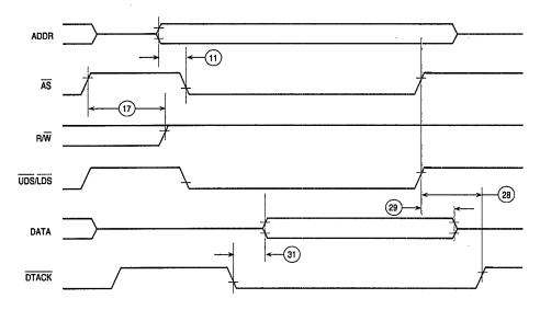
Figure 5-33. Pseudo-Asynchronous Read Cycle
