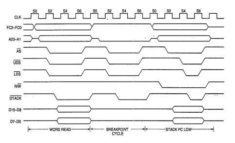
Figure 5-12. Breakpoint Acknowledge Cycle Timing Diagram
