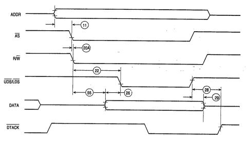
Figure 5-34. Pseudo-Asynchronous Write Cycle
