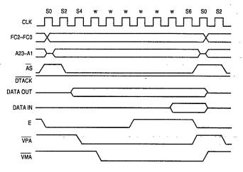
Figure B-4 M6800 Peripheral Timing—Best Case
