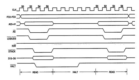
Figure 5-29. Halt Operation Timing Diagram
