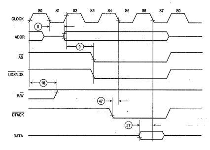
Figure 5-35. Synchronous Read Cycle
