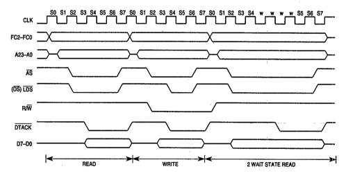
Figure 4-2. Read and Write-Cycle Timing Diagram
