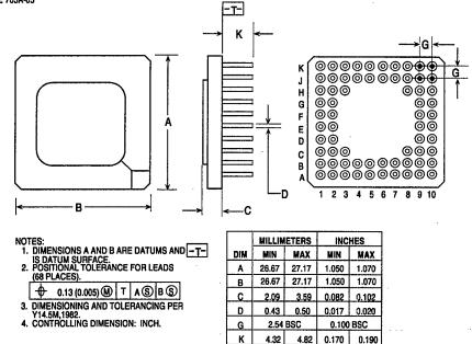
R SUFFIX PIN GRID ARRAY WITH STANDOFF (Dimensions essentially those of Case 765A-05.)
