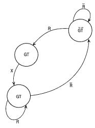
(b) 2-Wire Bus Arbitration Figure 5-18. Bus Arbitration Unit State Diagrams
