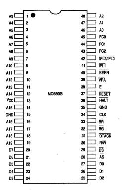
Figure 11-5. 48-Pin Dual In Line
