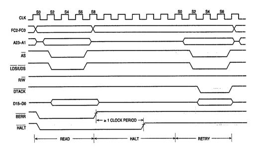
Figure 5-27. Retry Bus Cycle Timing Diagram
