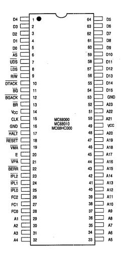
Figure 11-1. 64-Pin Dual In Line
