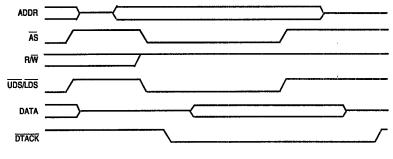
Figure 5-31. Fully Asynchronous Read Cycle
