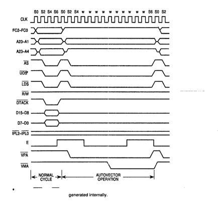
Figure B-6. Autovector Operation Timing Diagram
