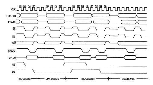
Figure 5-16. 2-Wire Bus Arbitration Timing Diagram
