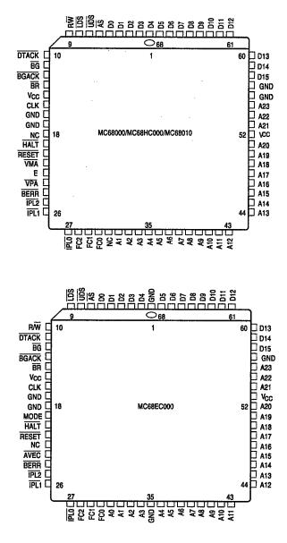
Figure 11-3. 68-Lead Quad Pack (1 of 2)
