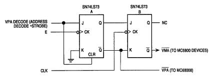
Figure B-2. Example External VMA Circuit
