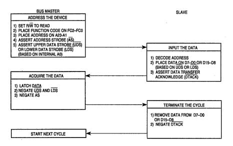
Figure 5-2. Byte Read-Cycle Flowchart
