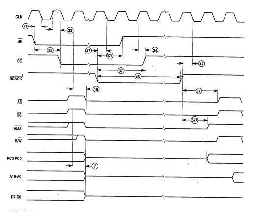
NOTE: Waveform measurements for all inputs and outputs are specified at: logic high 2.0 V, logic low = 0.8 V. 1 MC68008 52-Pin Version Only.
