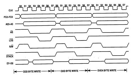
Figure 4-4. Write-Cycle Timing Diagram
