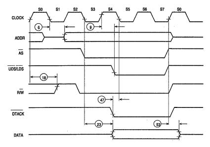
Figure 5-36. Synchronous Write Cycle
