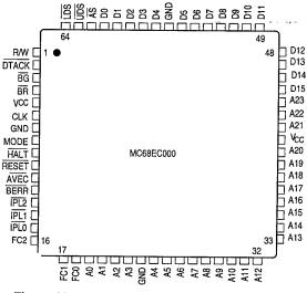
Figure 11-6. 64-Lead Quad Flat Pack-FU Suffix
