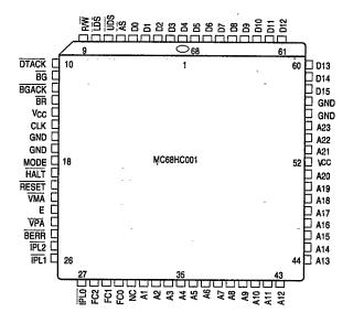
Figure 11-3. 68-Lead Quad Pack (2 of 2)
