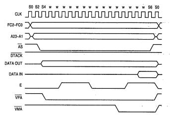
Figure B-5. M6800 Peripheral Timing—Worst Case
