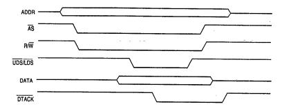
Figure 5-32. Fully Asynchronous Write Cycle
