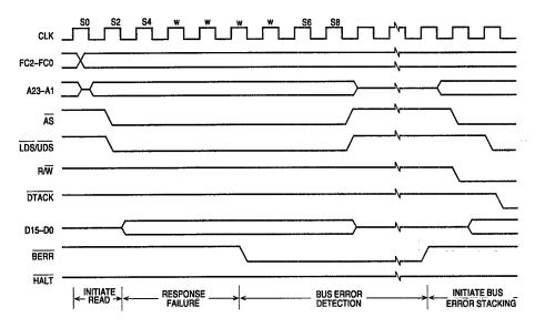
Figure 5-25. Bus Error Timing Diagram
