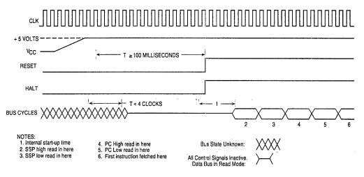
Figure 5-30. Reset Operation Timing Diagram
