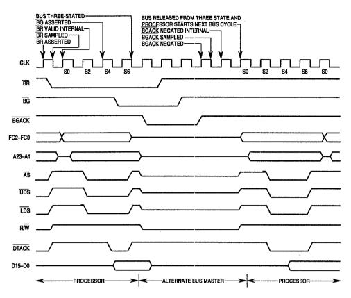
Figure 5-21. 3-Wire Bus Arbitration Tirning Diagram-Special Case
