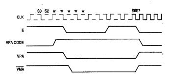
Figure B-3 External VMA Timing
