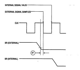
Figure 5-17. External Asynchronous Signal Synchronization
