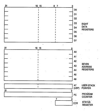
Figure 2-1. User Programmer's Model (MC68000/MC68HC000/MC68008/MC68010)
